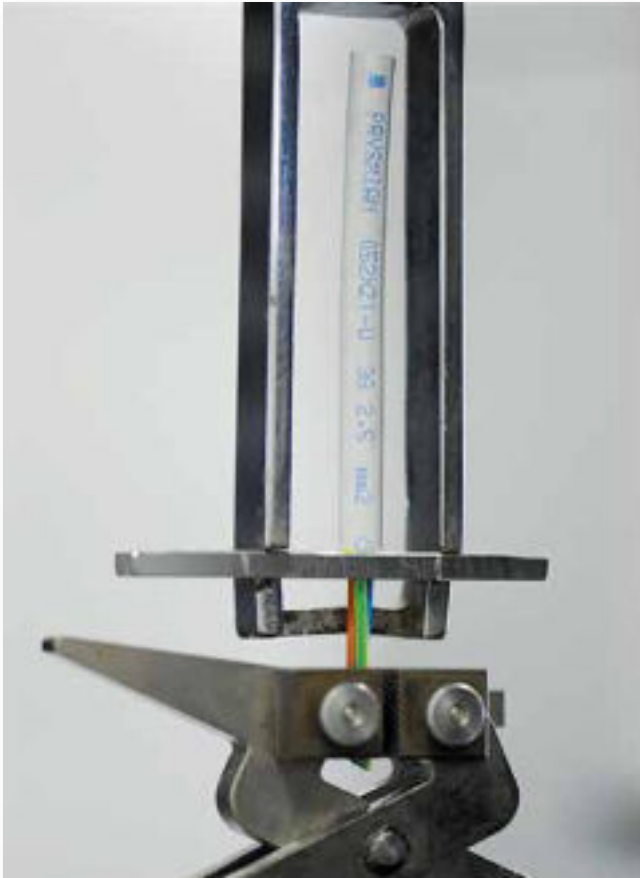
A cable sample in the stripping test.
