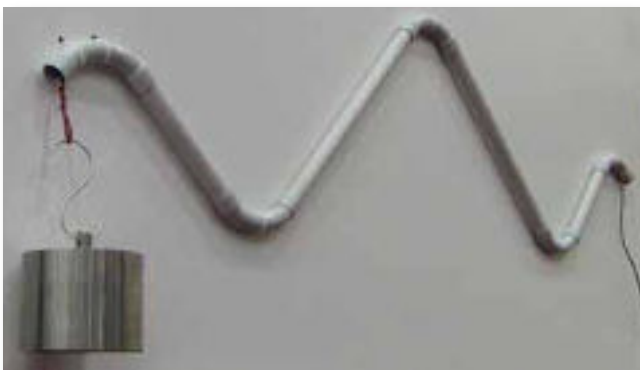
A cable sample in the slickness test.
