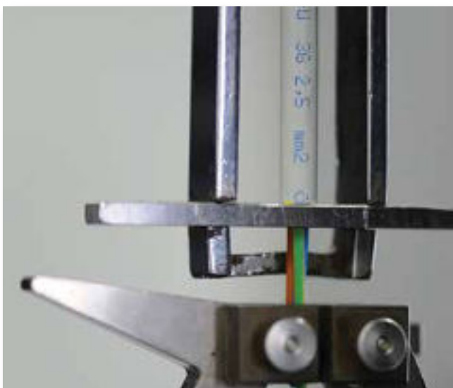
A sample in the stripping test.
