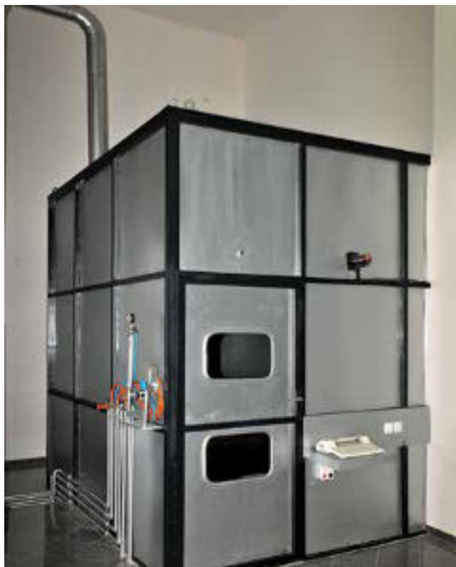
Smoke density testing cabin.
