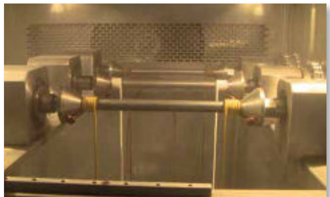
Cable samples in a cyclic strength test.
