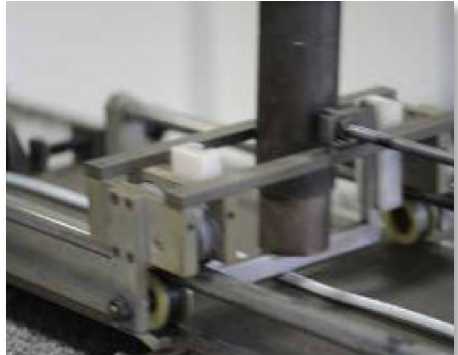
A cable sample in the abrasion test.
